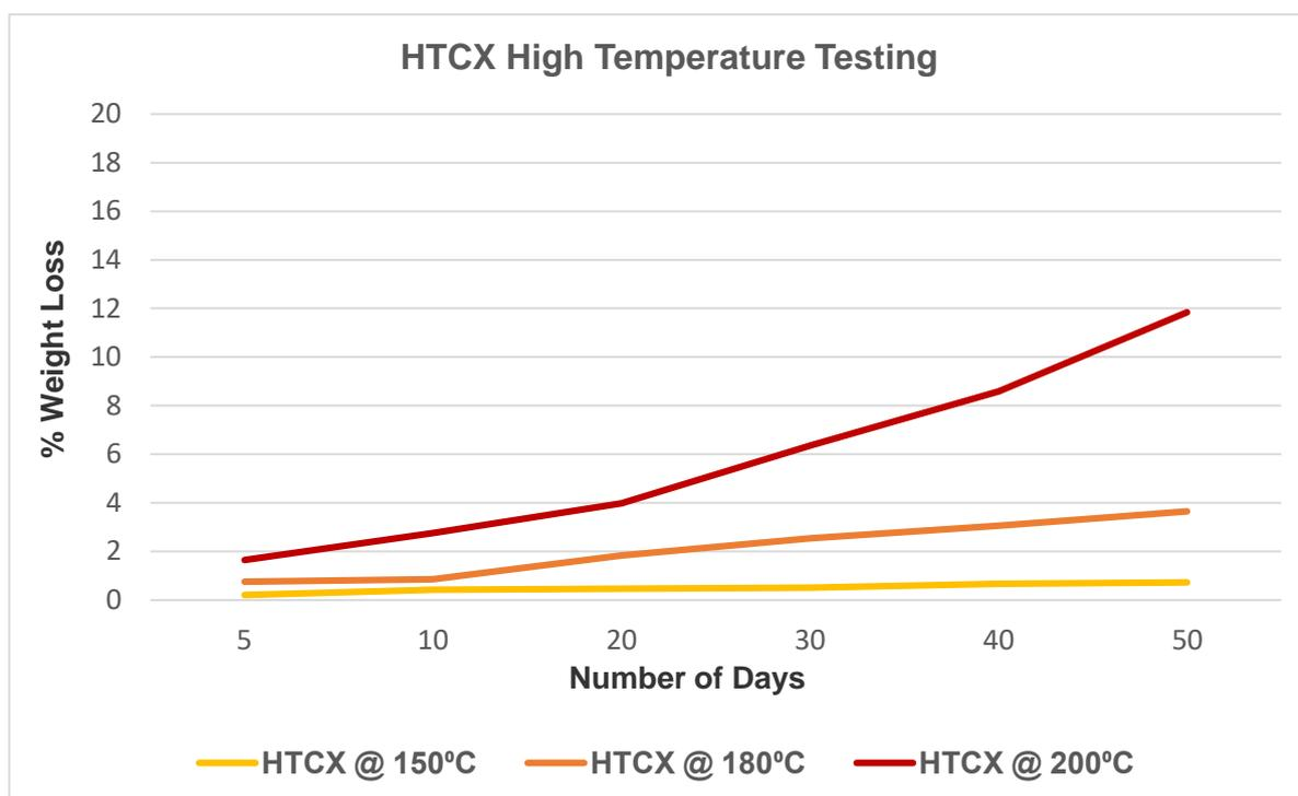
The above graph is provided for guidance only; testing in application conditions is advised. Tests were conducted 'open cup' therefore enhancing the weight loss effect. Tests conducted under in-use conditions may produce significantly lower results.
